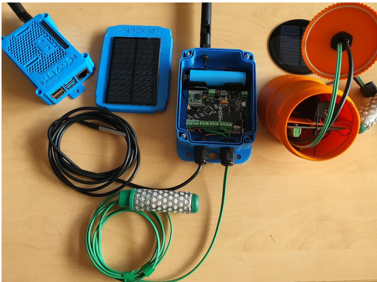
Figure 1: WaziGate (left), WaziSense that can be mounted to a pole (middle), WaziSense to be mounted inside pipe
