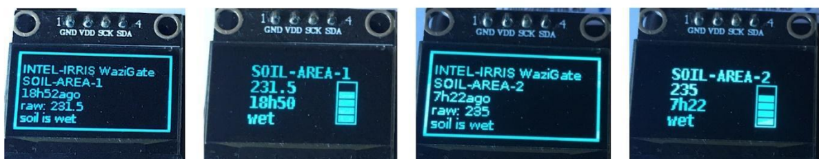
Figure 1: The OLED interface of the INTEL-IRRIS WaziApp on the WaziGate [1]
