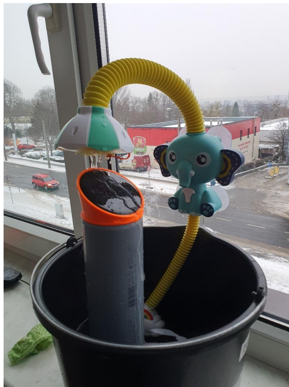
Figure 4: Rudimentary, preliminary Waterproof testing for the case in an ensembled condition
